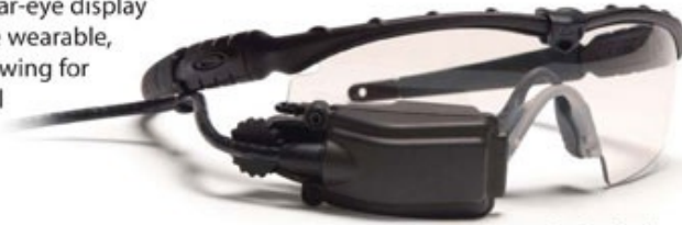
Tac-Eye Series Durable monocular head-mounted computer or video displays designed to clip onto safety glasses, headsets or safety goggles.
