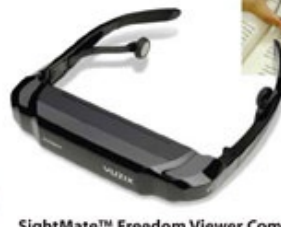
SightMate™ Freedom Viewer Combo iWear® AV920 video eyewear combined with a third-party handheld electronic magnifier helps individuals with impaired vision read small print.
